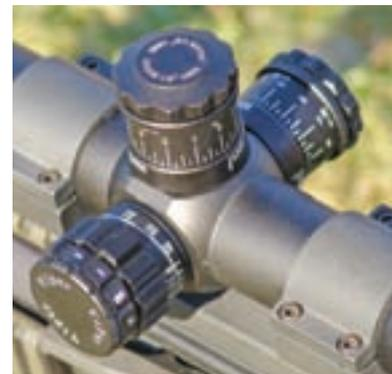
Detail of the Viper's saddle, the turrets are easy to dial and can be locked in position, on the left is a combined side focus and rheostat
